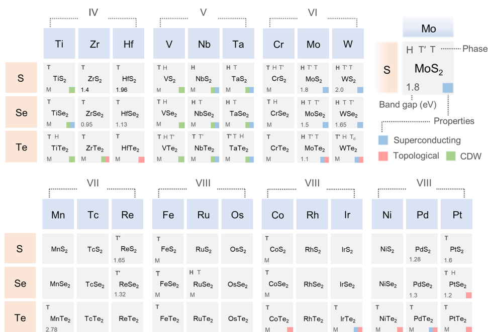
Figure 3. Periodic table of known experimentally synthesized layered TMD materials (groups IV, 64–77 V, 78–99 VI, 2,100–102 VII, 59,60,103,104 and VIII 105–125 ), summarizing their existing structural phases (H: trigonal prismatic, T: octahedral, T': distorted octahedral, T d : orthorhombic), typical band gaps (values at the bottom left corner of each grid, M: metallic), and observed electronic phases (superconducting, topological, and CDW).
